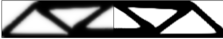
Figure 2-2: A symmetric topology optimization problem is shown with the filtered variable to the left and the projected variable to the right.
