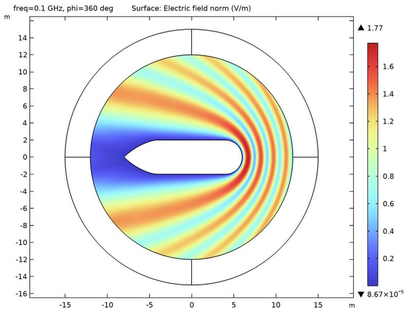
The default plot shows the norm of the total electric field for an angle of incidence equal to 360 degrees. The total electric field is the actual, measurable, physical field. The plot is dominated by a standing wave pattern caused by the reflections mainly on the stern
