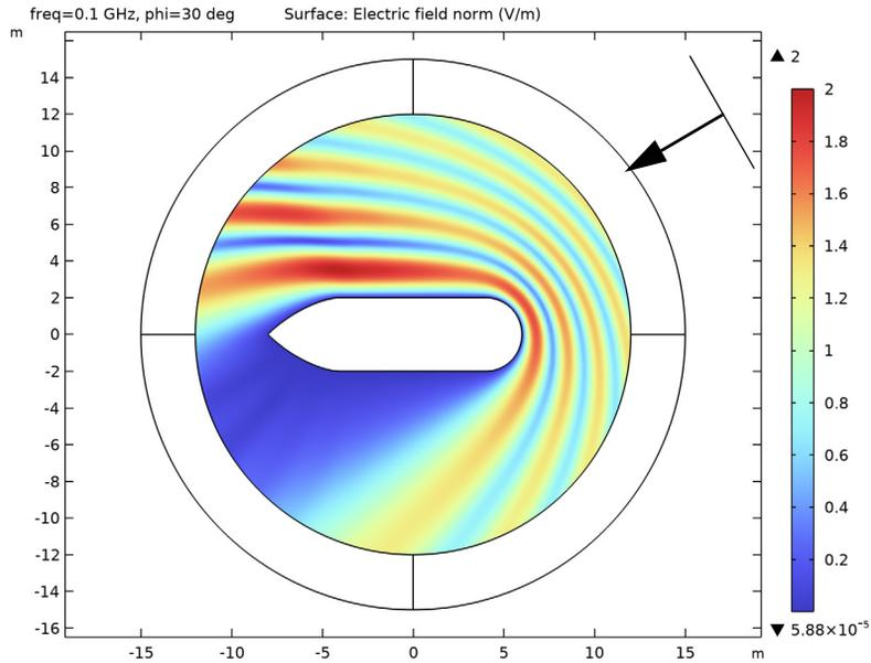
*Figure 2: The total field norm for a 30 degree angle of incidence. The arrow represents the propagation direction of the incident background field.*
