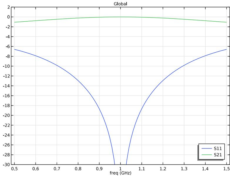
Figure 3: Spectral response for the transmission line. Notice that the transmission coefficient ( $S_{21}$ ) peaks at the frequency (1 GHz) for which the transformer is a quarter-wave long. At that frequency the reflection coefficient ( $S_{11}$ ) is zero (approaches negative infinity which the dB scale used in the graph).
