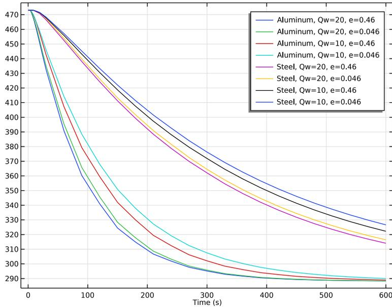
Figure 8: Average temperature of the polyurethane part as function of time and cooling conditions.
