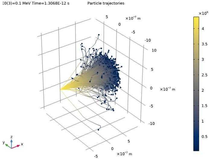
Figure 1: Trajectories of 0.1 MeV protons in silicon. The changes in direction are due to collisions with target nuclei. The continuous decrease in energy is from ionization loss.
