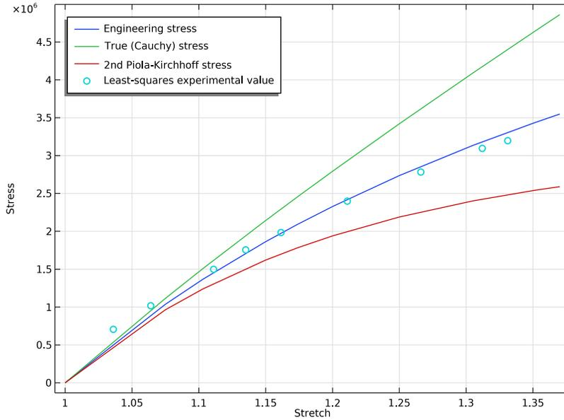
Figure 1: Measured (turquoise circles) and computed (blue line) engineering stresses. In addition, two other stress measures are plotted for comparison.
