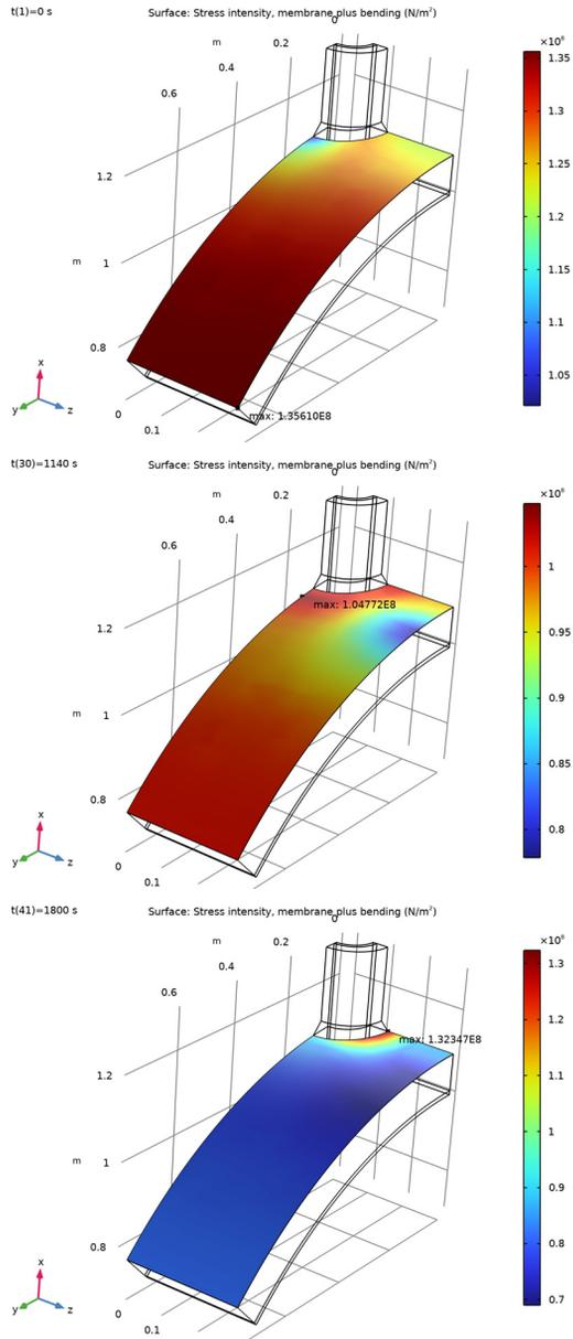
Figure 5: Membrane plus bending stress intensity at initial time (top), 1140 s (middle), and 1800 s (bottom).
