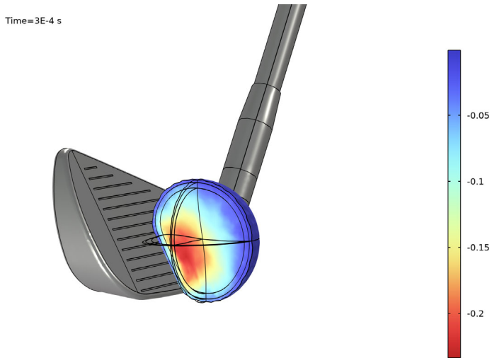
Figure 3: Deformation of the golf ball and distribution of the third principal (compressive) strain in the interior part of the ball at 0.3 ms.
