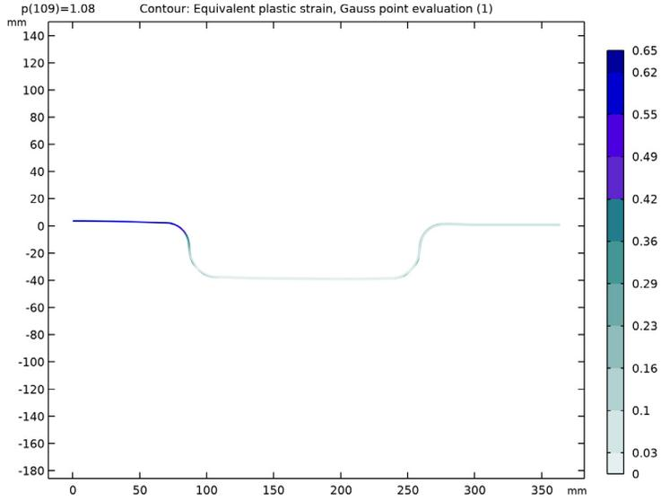
Figure 4: Plastic strains after release of the punch.
