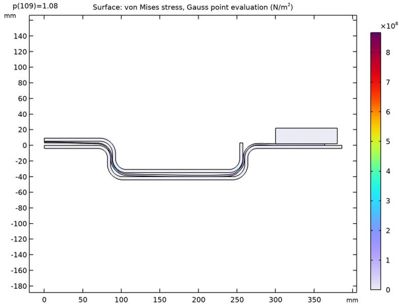
Figure 3: Residual stress after release of the punch.
