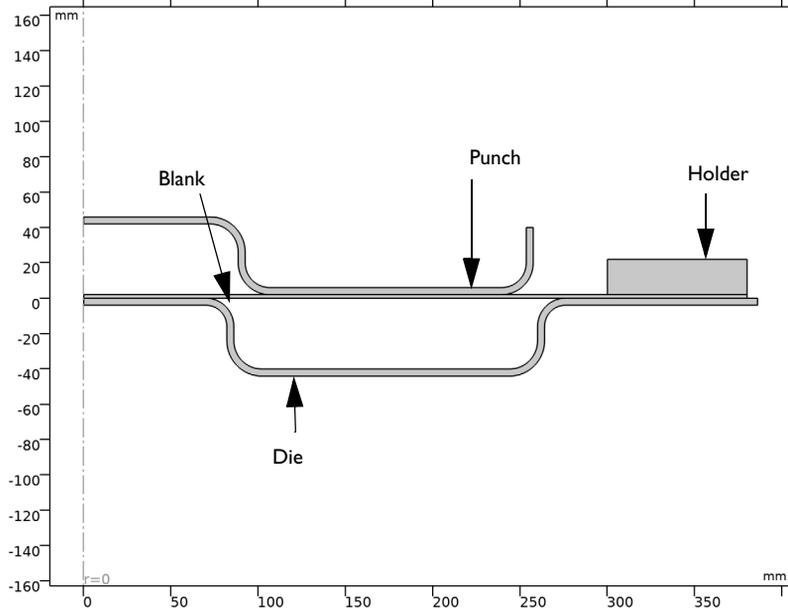
Figure 2: Forming tools setup.
