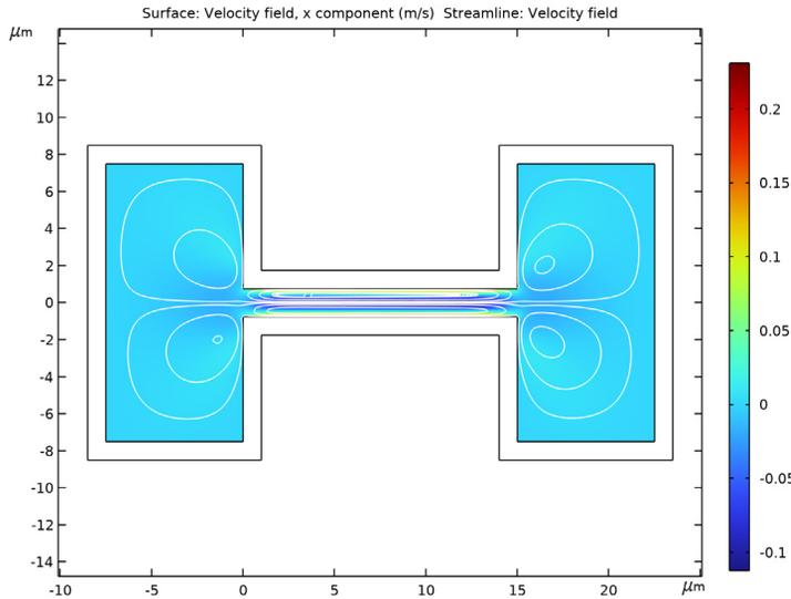
Figure 3:  $x$ -velocity (color) and streamlines (white) inside the channel. Flow is driven by thermal creep along the walls of the channel but a back-flow, driven by the pressure difference between the reservoirs, occurs in the center of the channel.
