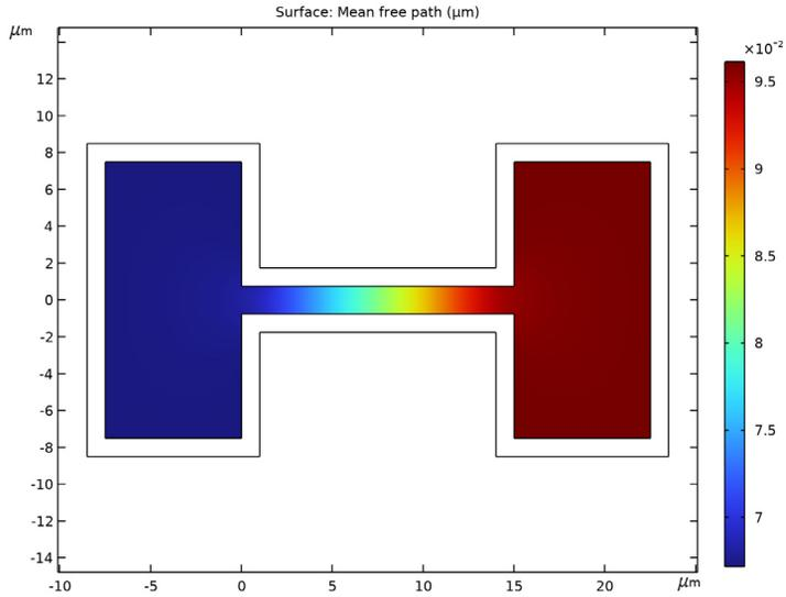
Figure 2: Gas mean free path. The channel width is  $1.5 \mu\text{m}$ , so the Knudsen number varies between 0.064 and 0.045.
