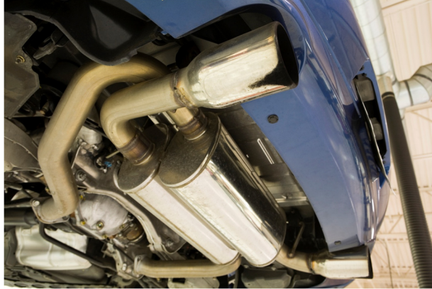
Figure 1: Catalytic converters reduce the NOx levels in the exhaust gases emitted by combustion engines.
