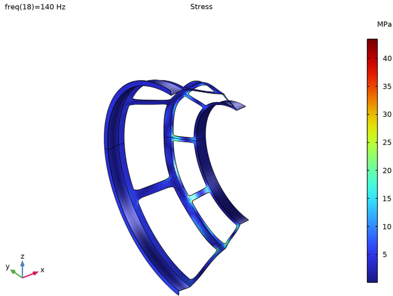
Figure 9: Stress distribution at 140 Hz on the basket.
