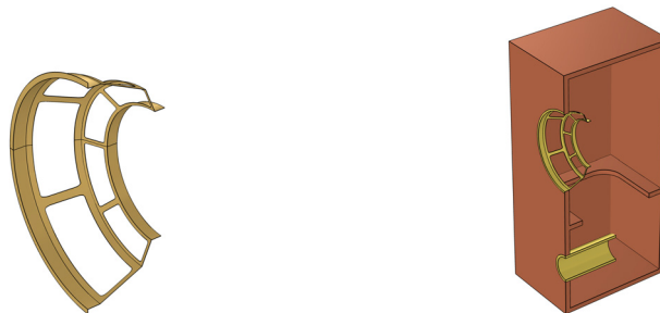
Figure 2: The basket (left) and the vented enclosure with basket and vent (right).
