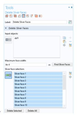
deleted you can edit the settings for the operation to set a tolerance that is just slightly larger than the width of the face.
