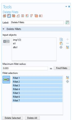
5 Seven fillets are found by the tool. These appear in the Fillet selection list, and they are also highlighted on the geometry.
