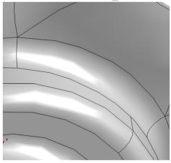
7 In the Settings window for Ignore Edges select the Activate Selection toggle button, then find some of the edges on the geometry by using Zoom to Selection All edges in the list are next to sliver faces, similarly to the image displayed to the right. The sliver faces are wider compared to those that were collapsed in the previous operation. The faces on the two sides of the edge are continuous across the edge, and it is thereby suitable to form a larger composite face by ignoring the edge.
