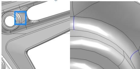
Both small faces and sliver faces are removed in this operation. Small faces with sides that are similar in length are usually collapsed into a vertex, whereas sliver faces that have a high aspect ratio are more often collapsed into one of the longer edges. As an alternative to the Collapse Faces operation you can also use the *Merge Edges* operation that gives more control over which edges are kept when collapsing faces.
