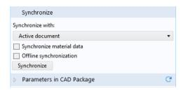
By this action you transfer the geometry of the pacemaker electrode from SOLIDWORKS to COMSOL.
