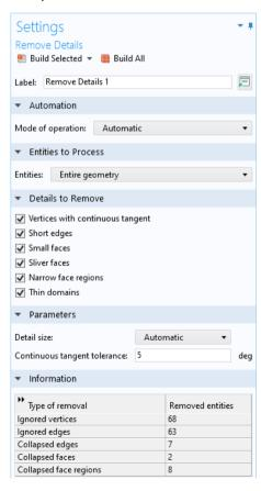
The fastest way to determine if this is the case is to build the mesh and check if the mesher displays any Information about small entities.
