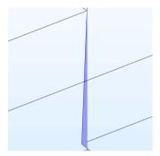
A sliver face is a face with a high aspect ratio. If it is not removed from the geometry it may cause problems during meshing. Remaining sliver faces in the list are located on the bezel of the flat screen TV, and some other on the two couches.
