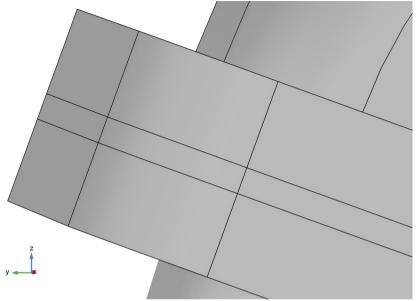
The thin domain is automatically detected and removed by Remove Details.
