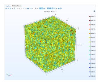
**Note:** The function conductivity has been evaluated again in MATLAB to generate the above plot. As the function is using a random distribution, the above plot does not exactly represent the distribution of the thermal conductivity when the solution has been computed.
