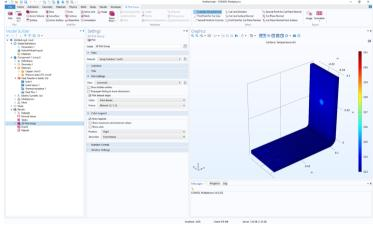
You may notice that the maximum temperature region is located in the bolt. To get a better rendering of the temperature distribution within the busbar, you need to change the color range.
