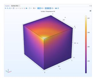
Visualize the material thermal conductivity on the geometry by adding a new 3D Plot group. In the Results tab, select 3D Plot Group 🛅 . An additional toolbar containing Plot Tools for the 3D Plot Group appears when the 3D Plot Group is selected in the Model Builder.
