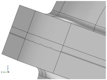
The gap between gasket and manifold is now eliminated, but there is still a slight overlap between the gasket and downpipe. Further ahead, you will delete the thin domain that results from the overlap by using *Remove Details*.
