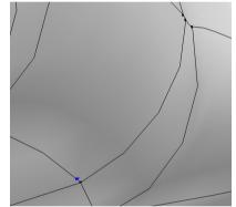
The sequence of virtual operations generated by Remove Details includes several other Ignore Edges and Ignore Vertices operations to remove slivers with increasing face width. In the following take a closer look at the *Collapse Face Regions* operation, that is added to the sequence to detect and remove narrow face regions.
