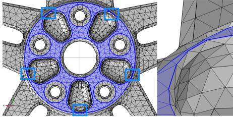
Since it is not easy to measure the width of a narrow face region without modifying the geometry, the fastest way to remove the narrow region is to manually increase the tolerance for Remove Details until the narrow regions are removed.
