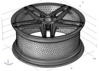
The generated mesh consists of approximately 68000 elements and there should be no Information nodes appearing under the Mesh 1 node due to small geometric entities.
