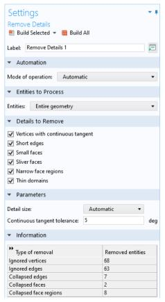
The fastest way to determine if this is the case is to build the mesh and check if the mesher displays any Information about small entities.
