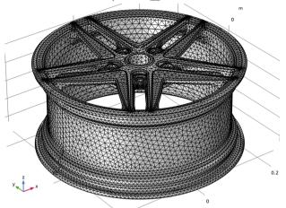
The generated mesh consists of approximately 68000 elements and there should be no Information nodes appearing under the Mesh 1 node due to small geometric entities.
