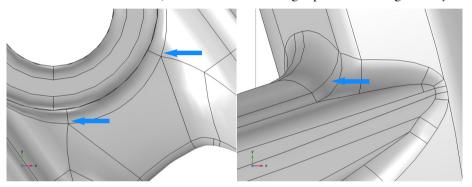
The small faces and slivers are no longer present in the geometry. According to the Information section in the Settings window for Repair, 60 short edges and 20 sliver faces were removed.
