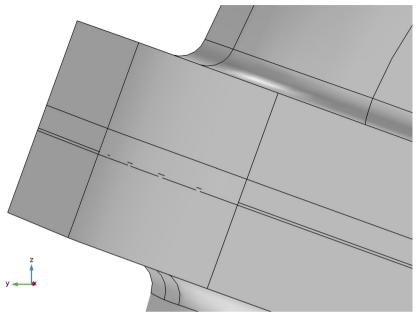
The gap between gasket and manifold is now eliminated, but there is still a slight overlap between the gasket and downpipe. Further ahead, you will delete the thin domain that results from the overlap by using *Remove Details*.
