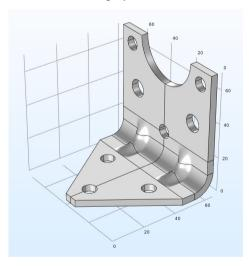
3 In the Model Builder expand Component 1>Geometry 1 to see the sequence of geometry operations that builds the bracket.
