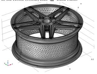
The generated mesh consists of approximately 68000 elements and there should be no Information nodes appearing under the Mesh 1 node due to small geometric entities.
