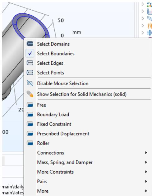
Figure 6-9: The context menu for adding a physics feature to the preselection (for Solid Mechanics).
