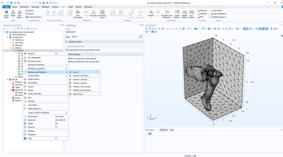
*Figure 8-9: The Model Builder context menu when clicking the Mesh node.*
