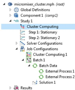
Figure 20-6: An example of the two kinds of Cluster Computing nodes available under Study and Job Configurations.
