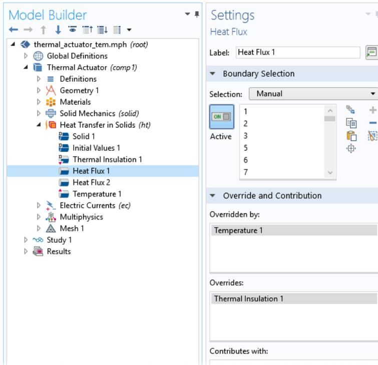
Figure 3-8: The *Override and Contribution* section lists other physics nodes that the selected node is overridden by, overrides, or contributes with.
