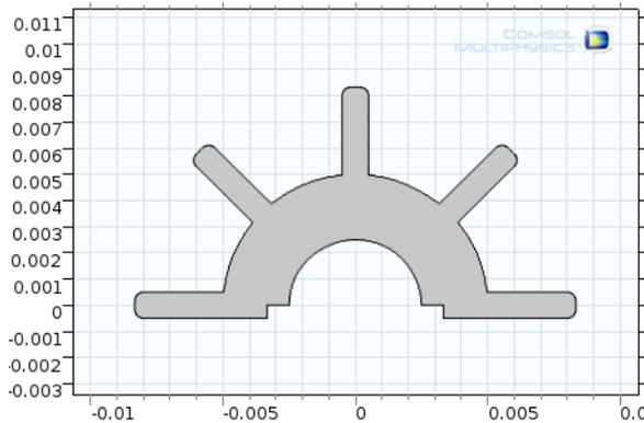
*Figure 7-49: Final 2D object created in the Model Builder.*
