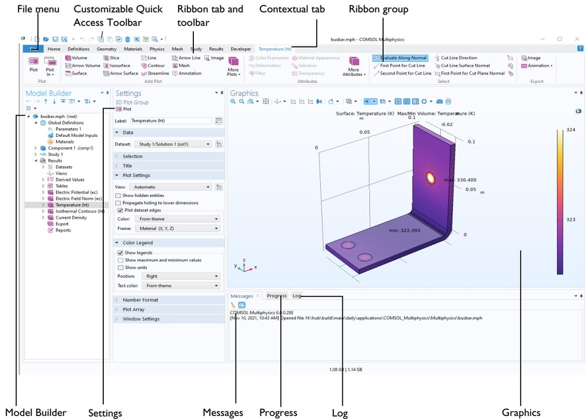
Figure 2-1: The default COMSOL Desktop with its major windows in a widescreen layout. The ribbon tabs and groups are available for Windows users. For macOS and Linux users the layout is similar but you access some options from the main menu or contextual toolbars.
