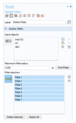
**5** Seven fillets are found by the tool. These appear in the Fillet selection list, and they are also highlighted on the geometry.
