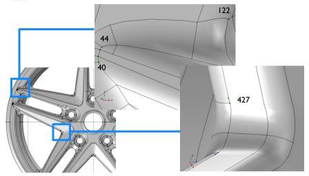
Three of these edges are located close to where the spokes connect to the rim, and one is found close to the center of the wheel. Similar edges occur on each spoke.
