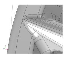
recommended to use a small tolerance together with the repair operation. If preserving the surface curvature is important for the analysis, virtual geometry operations, which work by hiding geometry features from the mesher, are available as an alternative. How you can do this is described further ahead, in the tutorial *Removing Small Geometric Entities Using Remove Details*.
