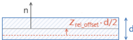
Figure 7-1: Meshed boundary indicated in red. The vector \mathbf{n} indicates the positive orientation of the boundary normal.
