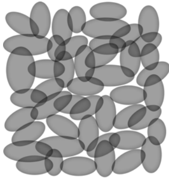
Figure 5-1: A block of a porous medium consisting of solids and the pore space between the solid grains. The average linear velocity describes how fast the fluid moves within the pores. The Darcy velocity attributes this flow over the entire fluid-solid face.
