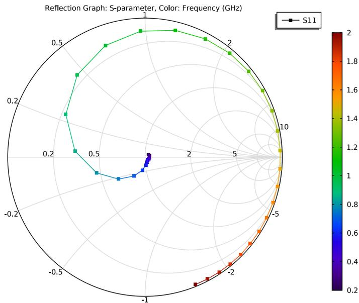
Smith plot showing the reflection coefficient  $S_{11}$ . The color legend shows the frequency, ranging from 0.2 GHz to 2 GHz.
