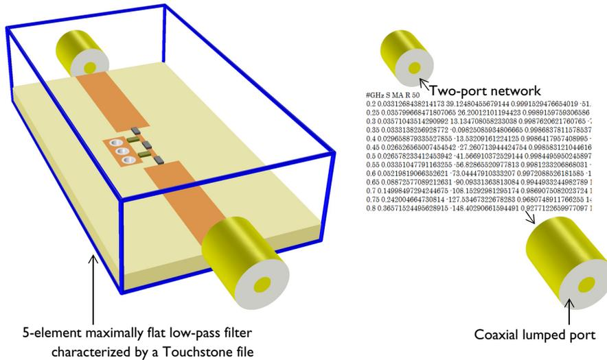
Figure 1: The circuit geometry inside a blue box frame is not included in the model but characterized by a Touchstone file.
