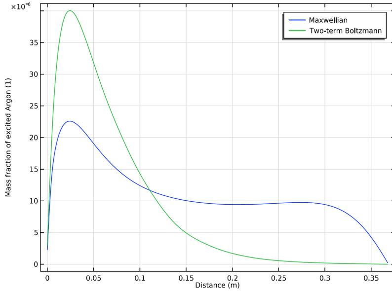
*Figure 5: Mass fraction of the excited argon obtained with the present model that computes the EEDF and from the same model where the EEDF was assumed to be Maxwellian.*
