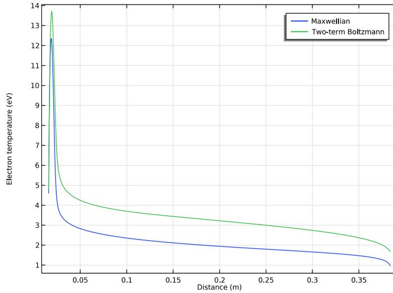
*Figure 3: Electron temperature obtained with the present model that computes the EEDF and from the same model where the EEDF was assumed to be Maxwellian.*
