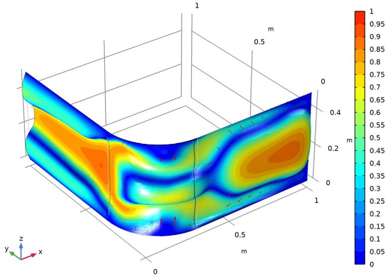
*Figure 2: The default shape optimization plot shows the edges of the old geometry in gray together with a surface plot of the relative normal boundary displacement in colors. The actual displacement is shown with red arrows.*
