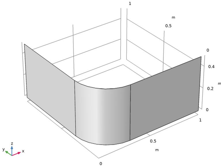
*Figure 1: The initial geometry is shown. The load is applied in the y-direction on the rightmost edge, while the displacement and rotation is fixed at the leftmost edge of the shell. The shape deformation of this edge is restricted to the  $xz$ -plane.*
