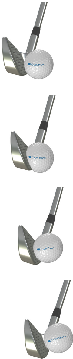
Figure 2: Snapshots of the club and golf ball during the simulation. From top to bottom, the timings are 0 ms, 0.15 ms, 0.30 ms and 0.45 ms.
