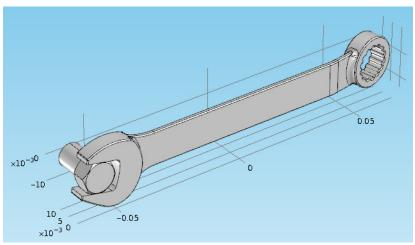
The bolt's fixed constraint is at the cross section shown below. A load is applied at the box end of the combination wrench.
