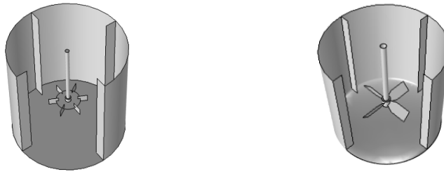
Figure 1: A baffled flat bottom mixer with a Rushton turbine (left) and a baffled dished bottom mixer with a pitched four blade impeller (right).
