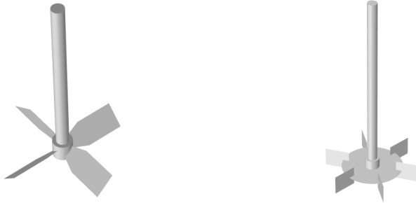
Figure 3: A four-blade pitched impeller (left) and a six-blade Rushton disc turbine (right).
