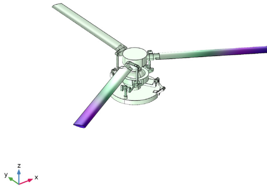
Figure 12: Mode shape of the helicopter swashplate mechanism (bending mode).
