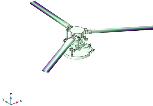
Figure 13: Mode shape of the helicopter swashplate mechanism (torsion mode).
