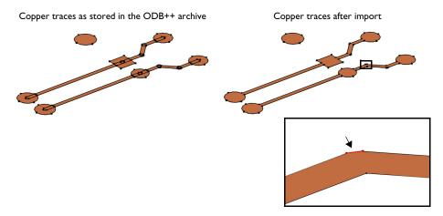
During import of the copper layers the individual shapes are united and the internal edges are removed to reduce the complexity of the geometry. The final geometry objects for the copper traces are shown to the right in the figure above. The short edge, which is highlighted above in the magnified section of the copper trace, is a result of two overlapping copper lines.
