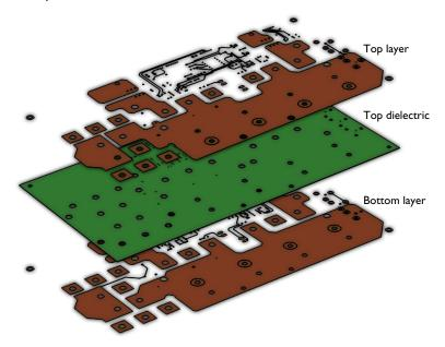
During import, geometry objects are generated for the copper layers (surface objects), the dielectric layer (solid object) and vias (solid objects). The solid object for the dielectric layer is created according to the shape of the board as defined in the ODB++ archive. The vias are generated as solid cylinders. To get the geometry for simulation, the objects for the dielectric material are united with the copper surface objects, and the cylinders for the vias are subtracted from the result.
