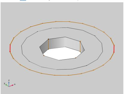
The highlighted edge is one of the segments of a polygon that represents a circular edge in the top copper layer. Such polygons can occur often in PCB data, and are one of the sources for short edges in the generated geometry.
