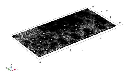
According to the information in the **Messages** window, the mesher generated a mesh of approximately 130000 domain elements, and also resulted in four warning nodes. Proceed with reviewing these warnings to get an insight into the various issues associated with meshing this PCB geometry.
