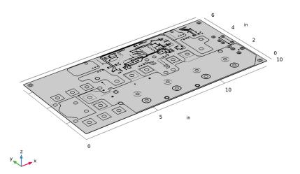
Due to the high aspect ratio of the imported geometry it is not possible to see the vias that are inside the dielectric. To make this possible create a second view.
