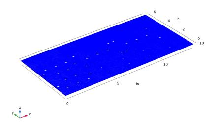
This final mesh has approximately 265,000 domain elements. Warnings are no longer displayed by the mesher as the applied maximum and minimum element size parameters are now much closer to the size of the small details of the geometry.
