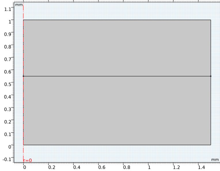
Figure 3: Axisymmetric model geometry.
