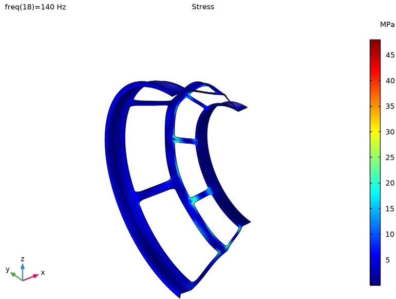
Figure 9: Stress distribution at 140 Hz on the basket.
