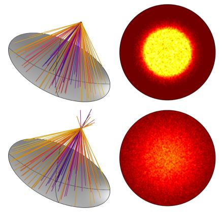
Rays released from an illuminated solar reflector and resulting concentration ratios in the focal plane. The top row is the ideal case. The bottom row includes surface roughness and solar limb darkening effects.
