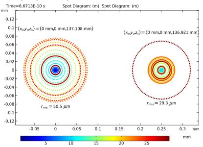
The double Gauss lens spot diagram. On the left is the spot on the nominal image surface. The spot on the right is located at the "best focus" image plane that has been computed automatically.
