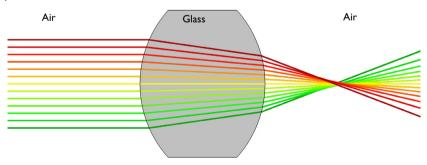
Ray propagation through a lens with a homogeneous (non-graded) index.
