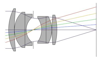
Overview of a double Gauss lens. In this view the marginal rays of an on-axis trace are shown, together with the chief ray of 4 additional fields.
