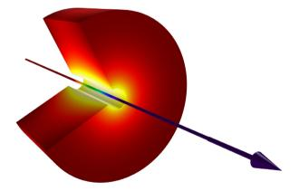
A ray passes through a layer of absorbing material, causing the temperature in the layer to increase.
