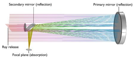
A simple Newtonian telescope. The incident rays are focused by a parabolic primary mirror and then redirected to the focal plane by a flat secondary mirror.
