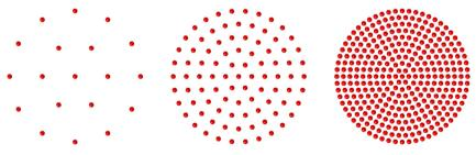
The hexapolar grid. From left to right, these grids have 2, 5 and 10 radial rings respectively. The number of rays launched would be 19, 91, and 331 in each case.
