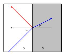
Refraction of an incident ray (blue) at a boundary. A second, reflected ray (red) is also released.
