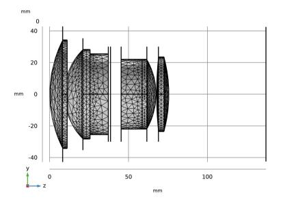
The default Physics-controlled mesh for the double Gauss lens.
