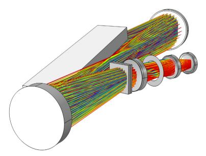
Ray diagram of a white pupil echelle spectrograph, which uses a combination of an echelle grating operated at high order and a cross dispersion grating operated at low order to separate light by wavelength. The light is then focused by a Petzval lens system.
