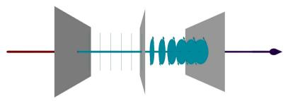
Linear Wave Retarder tutorial: An unpolarized ray (going left to right) passes through a linear polarizer, a quarter-wave retarder, and a second linear polarizer orthogonal to the first. Polarization ellipses are shown in the ray diagram. The color expression indicates the ray intensity.
