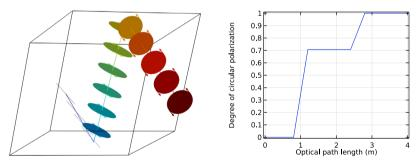
Linearly polarized light is internally reflected twice in a Fresnel rhomb (left). As a result, the ray's polarization ellipse shifts from linear, to elliptical, to circular. This can also be shown by plotting the degree of circular polarization plotted as a function of optical path length (right).
