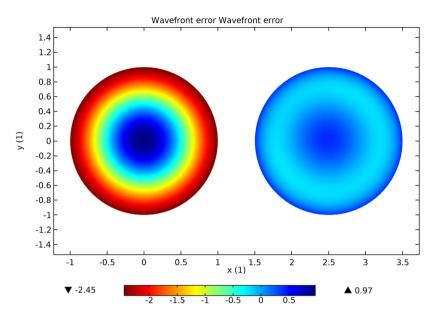
The double Gauss lens optical aberration diagram. The plot on the left uses all Zernike terms. In the plot on the right, the piston and defocus terms have been removed. Spherical aberration dominates the remaining terms.
