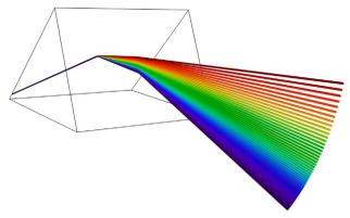
A prism containing a dispersive medium can separate light into different colors.
