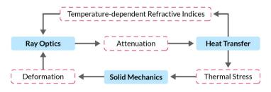
Bidirectional (two-way) coupling between ray optics and heat transfer, including thermal stress.
