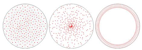
Release positions based on the domain mesh (left), nonuniform density expression (middle), and uniformly distributed along a boundary (right).
