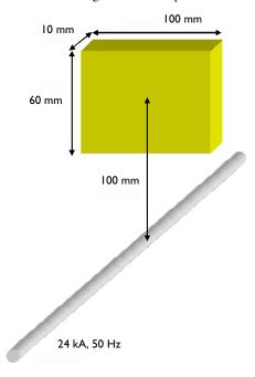
Because one cannot afford meshing an infinite volume, it is necessary to specify a finite volume to mesh and solve for. In this case, it makes sense to enclose the wire and the plate in a cylinder with the wire on the axis of this cylinder. This is a good choice when used with the default boundary condition, Magnetic Insulation. This condition forces the field to be tangential to the exterior boundaries. For the cylindrical shape of the domain that is a reasonable approximation to reality.
