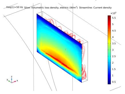
A total dissipated power of 6 W was obtained from integration through the plate. If you repeat the simulation for different materials, the application shows that lowering the conductivity decreases the dissipated power. However, for high permeability materials like soft iron, the dissipated power is higher than in copper (27 W) despite a much lower conductivity.
