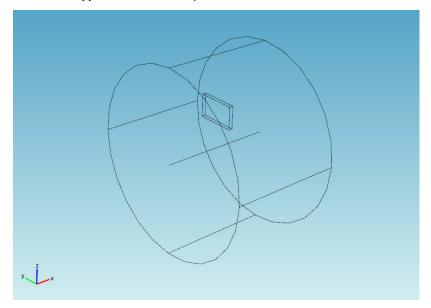
The conductor is modeled as a line current with 0° phase and an effective (RMS) value of 24 kA.
