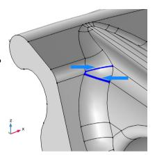
The visualization of the rim in the Graphics window is updated to reflect that the selected edges, and, where applicable, adjacent vertices are no longer part of the geometry which is going to be meshed.
