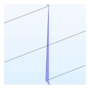
A sliver face is a face with a high aspect ratio. If it is not removed from the geometry it may cause problems during meshing. Remaining sliver faces in the list are located on the bezel of the flat screen TV, and some other on the two couches.
