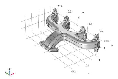
Rotate the geometry. As you can see it is hollow inside. As shown below, you can obtain the geometry for the inside in just one operation.
