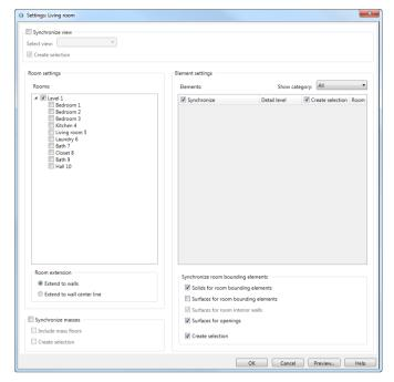
The Rooms list to the left contains the rooms defined in the project. To include the geometry of a room in the synchronization select its check box.
