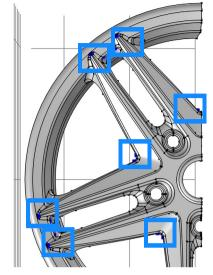
The resulting geometry is similar to the one after the last repair operation in the previous tutorial. The difference is that using the defeaturing tools you can have more control over which entities to delete and in which order.
