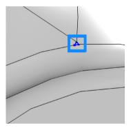
5 The new mesh contains fewer elements since the sliver and small face are no longer visible to the mesher.
