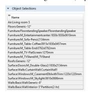
These selections are on the object level, and clicking on a selection in the table highlights the corresponding objects in the Graphics window. The selections are available for input to operations and settings during all stages of the model set-up. Read more about how to work with selections in the *COMSOL Multiphysics Reference Manual*.
