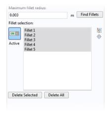
As the operation completes and the fillets are removed note that the Delete Fillets 1 (dfi1) node is inserted into the geometry sequence, just above the Cap Faces 1 (cap1) node. The Cap Faces 1 (cap1) node is still unavailable, meaning that it is currently not built.
