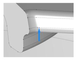
4 To mesh the geometry once more right-click the Mesh 1  $\triangleq$  node and select Build All  $\equiv$  .
