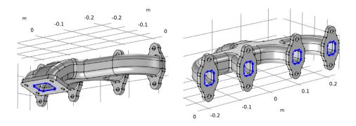
These edges can be selected directly in the Cap Faces operation, however a more efficient way, which only requires the selection of one segment from each edge loop, is to use an explicit selection where you have the option to automatically include continuous edges in the selection.
