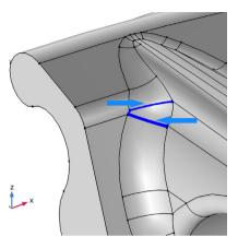
The visualization of the rim in the Graphics window is updated to reflect that the selected edges, and, where applicable, adjacent vertices are no longer part of the geometry which is going to be meshed.
