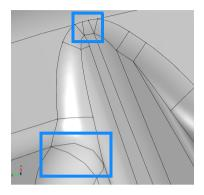
recommended to use a small tolerance together with the repair operation. If preserving the surface curvature is important for the analysis, virtual geometry operations, which work by hiding geometry features from the mesher, are available as an alternative. How you can do this is described further ahead.
