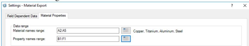
The properties are now listed in the table in the Material property settings section. You now need to assign valid COMSOL properties to the material properties in the spreadsheet.
