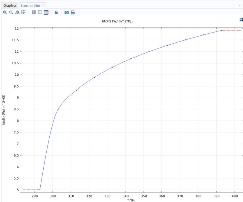
Now continue with changing the model settings to use the newly defined function for the heat transfer coefficient in the heat flux boundary condition.
