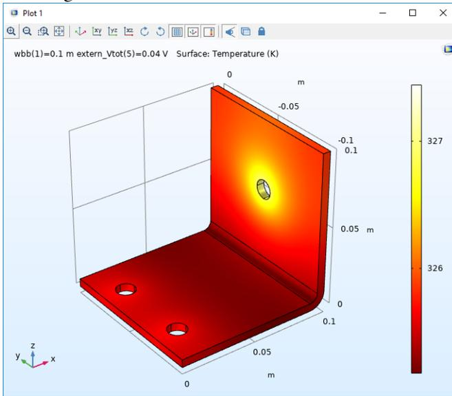
The plot represents the solution computed before the change of the busbar width.
