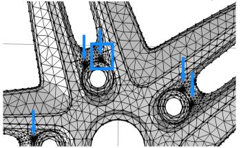
The areas of dense mesh, indicated by the arrows in the figure, are due to slivers and small faces. Zooming in even closer inside the blue rectangle reveals a small triangular face sitting adjacent to a sliver face. Two of these can be found around each bolt hole location. The edges that are highlighted in blue are listed in the Selection list of the Warning window.
