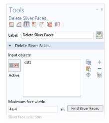
The tool removes sliver faces by collapsing them into an edge, and in this process it uses the tolerance specified for the search. For best results the tolerance needs to be close to the actual width of the face that is deleted. If it happens that a sliver cannot be deleted you can edit the settings for the operation to set a tolerance that is just slightly larger than the width of the face.
