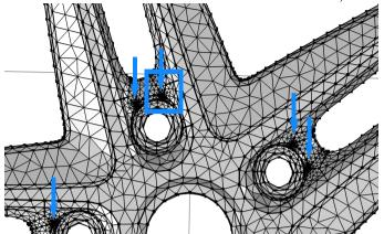
The areas of dense mesh, indicated by the arrows in the figure, are due to slivers and small faces.
