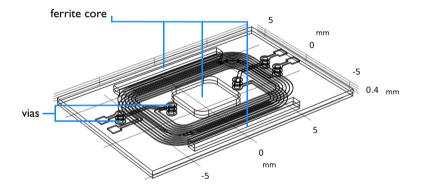
4 Switch to the Selection List window to view the generated objects. The import extrudes drill layers separately for each dielectric layer, and names these by combining the name of the drill and dielectric layers. For example the ferrite core, generated from the THROUGH.HOLES layer is extruded into two separate objects: THROUGH\_HOLES\_INNER\_LAYER\_DIEL and THROUGH\_HOLES\_TOP\_LAYER\_DIEL.
