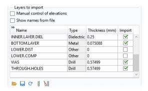
**Note:** When the file is scanned the elevation and thickness of drill layers is automatically detected. In this case the drill layers span both dielectric layers.
