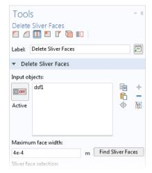
The tool removes sliver faces by collapsing them into an edge, and in this process it uses the tolerance specified for the search. For best results the tolerance needs to be close to the actual width of the face that is deleted. If it happens that a sliver cannot be deleted you can edit the settings for the operation to set a tolerance that is just slightly larger than the width of the face.
