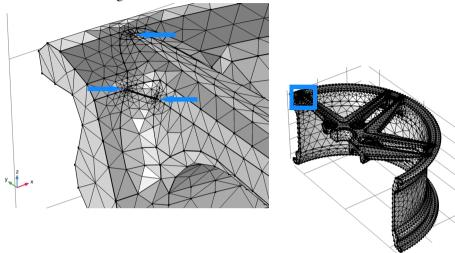
On closer examination you can see that several edges in this area are highlighted as being too short to be meshed with the current mesh settings.
