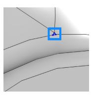
**5** The new mesh contains fewer elements since the sliver and small face are no longer visible to the mesher.
