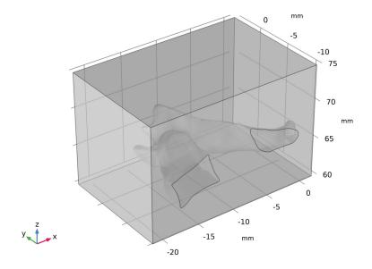
The resulting object now contains two domains, inside and outside the imported geometry. As a final step create a mesh for the geometry.
