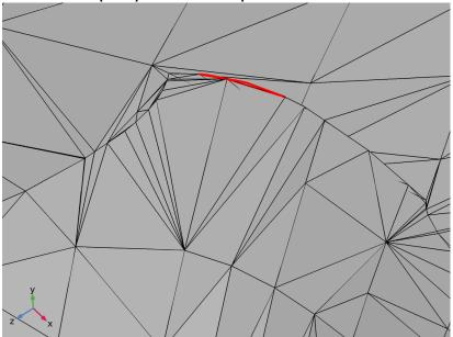
On the imported mesh Boundaries 4 and 5 are in the same location as the short edges on the generated geometry. These are isolated boundaries on the outside of the surface mesh, and are attached to the mesh only through a single edge. Isolated boundaries such as these are automatically removed during the last step of the geometry creation process, when the solid object is created.
