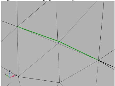
The two edges are located at the boundary of a small face that forms a fold in the geometry. To find where the two short edges originate from switch to the Mesh Part I sequence.
