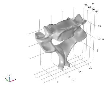
Notice that after the import completes you can no longer see the reference to the STL file in the **Settings** window. The source for the geometry import is now **Mesh Part 1**, which is where the mesh import can be found. The **Import 1** node in the geometry sequence handles the last steps of the process: conversion from mesh to geometry, and creation of a solid object.
