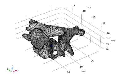
Two short edges, which are listed in the Warning I node that appears, have been detected.
