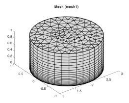
Figure 3-9: Extruded 3D prism mesh.
