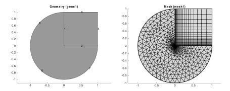
Figure 3-7: Incrementally generated mesh (right).
