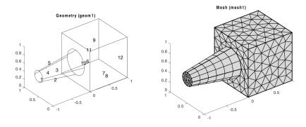
Figure 3-10: Combined structured/unstructured mesh.
