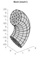
Figure 3-8: 3D prism mesh created with the Sweep feature.
