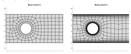
Figure 3-12: Initial unstructured quad mesh (left) and resulting boundary layer mesh (right).
