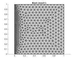
Figure 3-3: Refined mesh on boundary I(maximum element size = 0.02).
