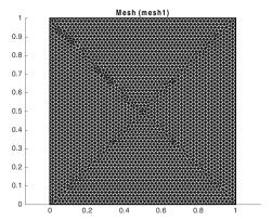
Figure 3-2: Fine mesh (maximum element size = 0.02).
