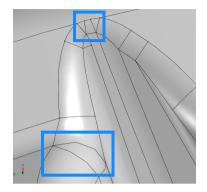
recommended to use a small tolerance together with the repair operation. If preserving the surface curvature is important for the analysis, virtual geometry operations, which work by hiding geometry features from the mesher, are available as an alternative. How you can do this is described further ahead.
