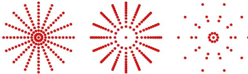
Figure 7-2: Comparison of the cylindrical release in which rays are positioned at uniform radius intervals (left), with uniform number density (center), or at user-defined radii (right).
