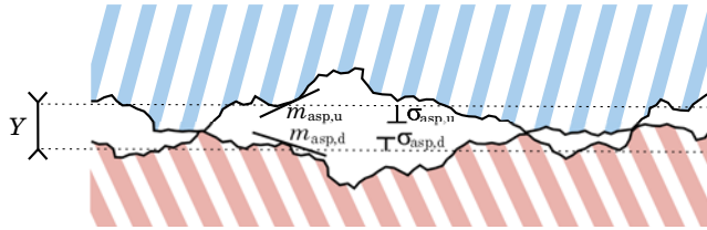
Figure 4-5: Contacting surfaces at the microscopic level.
