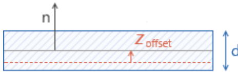
Figure 5-3: Meshed boundary indicated in red. The vector \mathbf{n} indicates the positive orientation of the shell normal.
