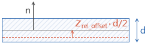
Figure 5-6: Meshed boundary indicated in red. The vector \mathbf{n} indicates the positive orientation of the shell normal.
