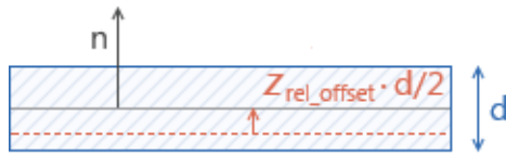
Figure 5-4: Meshed boundary indicated in red. The vector \mathbf{n} indicates the positive orientation of the shell normal.
