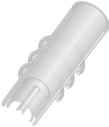
Figure 1: Geometry of an inductively coupled plasma torch. The torch is composed of three concentric quartz tubes in which gas are injected from the bottom and exit from the top the torch. In this model, a fixed power of 11 kW is transferred to the plasma by a three turn coil operating at 3MHz.
