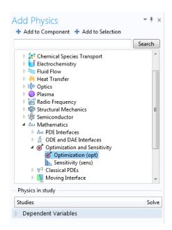
2 Click **Add to Component. Optimization** is added under the chosen Component in the Model Builder.
